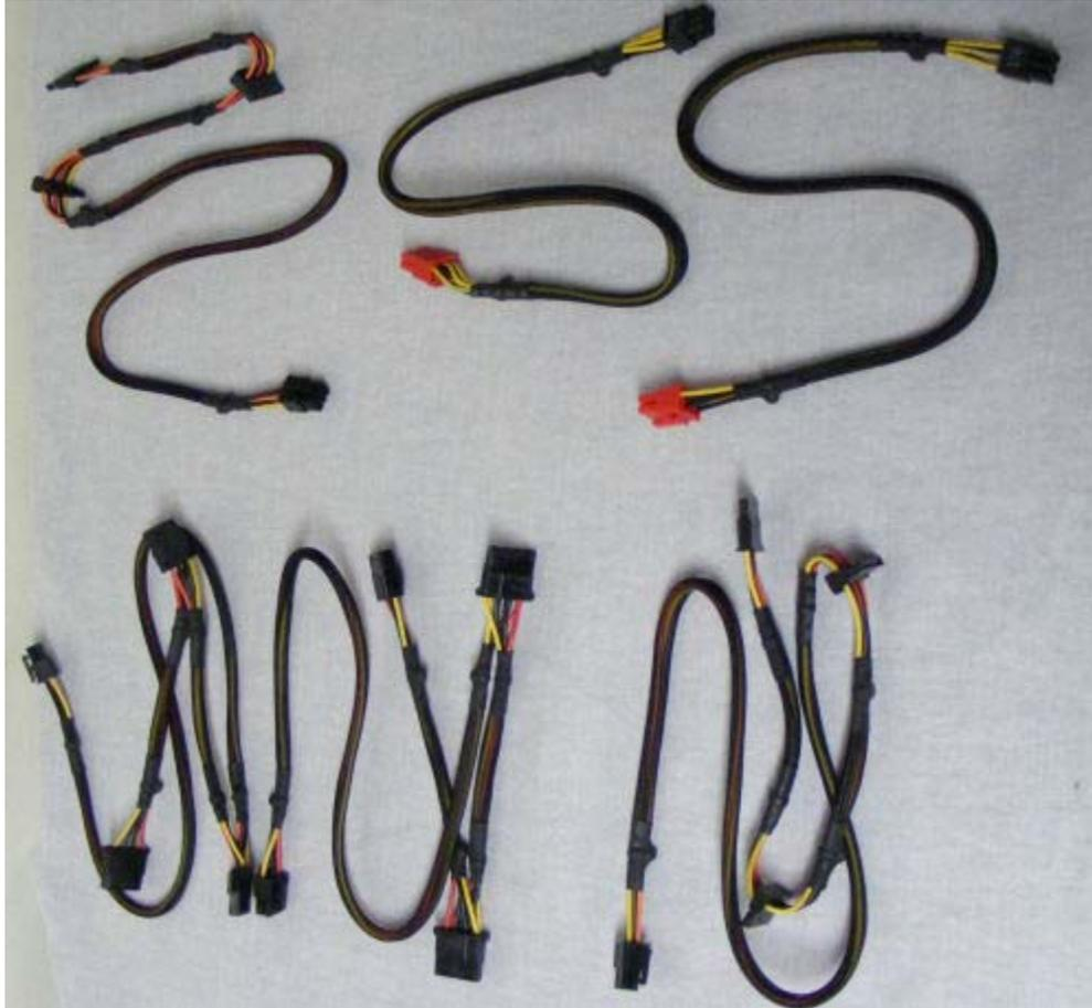
And here are the modular cables. Red connectors for the PCI-E cables, and black for everything else.
