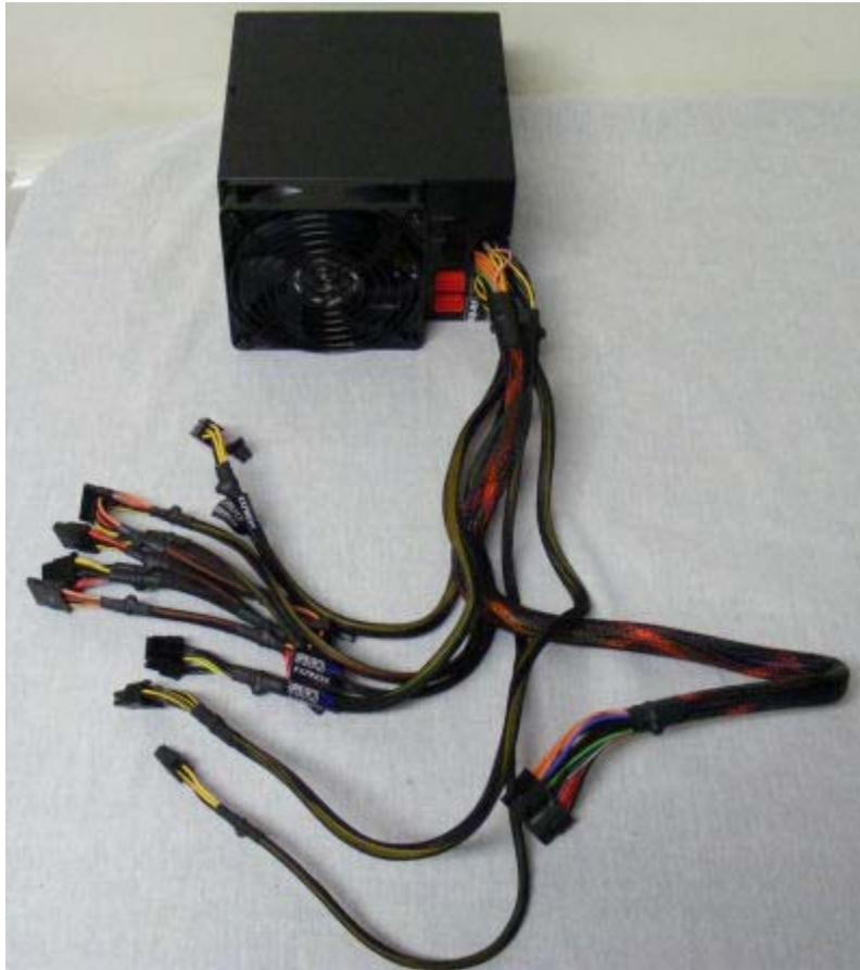
The tentacle shot kind of disappointed me for one reason above all others - Antec has seen fit to include both an ATX12V cable and an EPS12V cable. In addition to a single chain of Molexes and a single chain of SATA connectors. Again. Just like the [Truepower New](#). Come on, Antec, you made this thing modular, how about making the hardwired stuff less cluttered? This is going to cost a point or two again.
