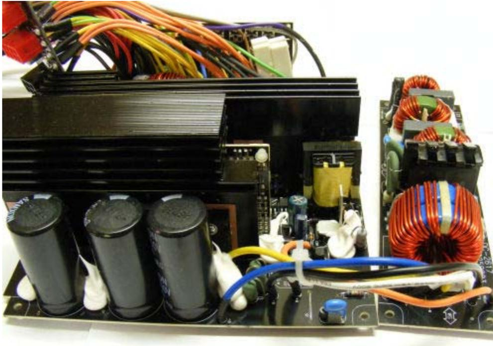
This is the primary side. Three big main filter capacitors from Samxon can be seen at the bottom of the pic. That big coil over there in the foreground on the transient filter board is the PFC coil.
