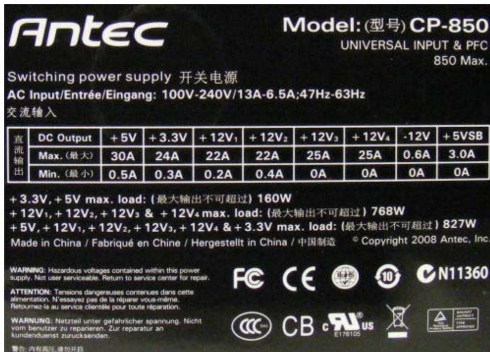
No clues to the OEM can be gleaned from the UL file number here, for it traces back to Antec. The hope that I might be dealing with a Signature in a big case increased when I saw this, for the 12V rails are rated identically. However, the 3.3V and 5V rails are not rated like an SG-850, so I'm still going to have to do my homework on page three. Also, the 12V combined rating is 1A lower on this model at 64A.
